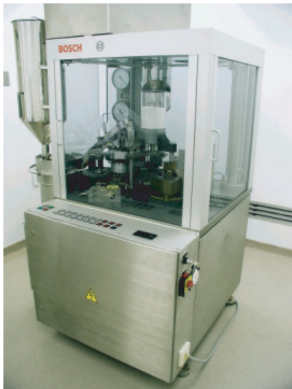
Figure 2. Photograph of production-scale machine for filling and sealing starch capsules.
